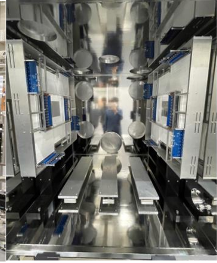
BDC (left) & SC (right) in beam diagnostic vacuum chamber
