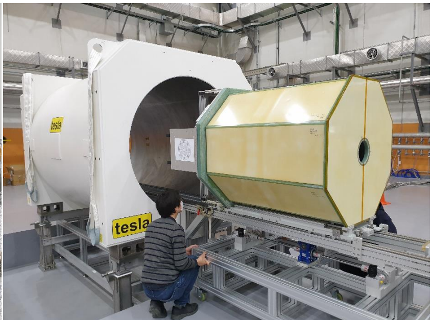
Installation of TPC inside the magnet
