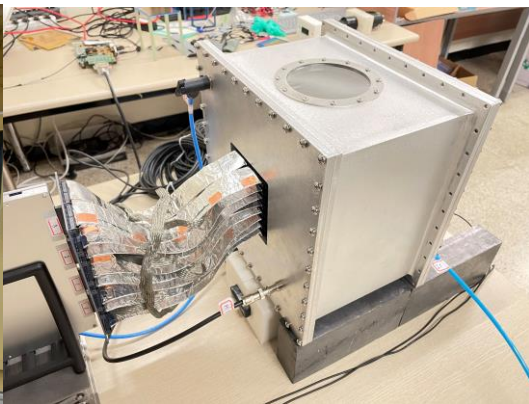
Low-energy detectors (Left) SC magnet ( B_{max} = 1.5 \text{ T} ) (Above) AT-TPC
